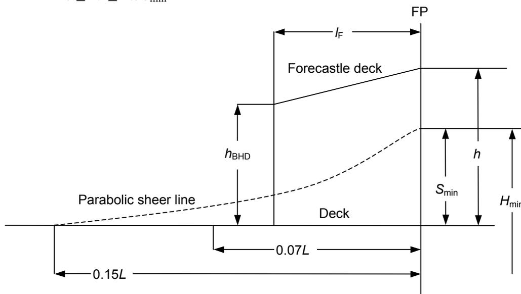
The height of the forecastle at the bulkhead position shall not be less than the ordinate, at that point, of a parabolic sheer curve having an ordinate S<sub>min</sub> at the
